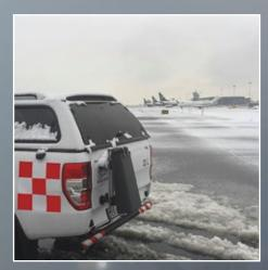
It is ideal to record the conditions on the entire runway, in terms of both length and width. Mobile sensors such as MARWIS can do this by installing several sensors on a unit behind the measuring vehicle.
