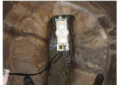
Web-Enabled DDS FLO-DAR AV Sensor in 18" Sewer Line in McKinney, TX
